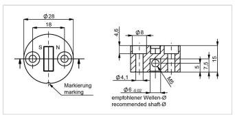
Position marker for frontal fixation with 2 cylinder head screws M4x20 (with screw lock) or with threaded pin M5 (both included in delivery). PF
