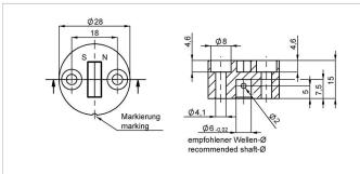
Position marker for frontal fixation with 2 cylinder head screws M4x20 (with screw lock) or with locking pin (both included in delivery).
