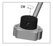
When the marking of the position marker is pointing away from the cable, the output is in the vicinity of the reference pulse (Z). Rotational direction CW: A leads before B.
