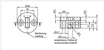
Position marker for frontal fixation with 2 cylinder head screws M4x20 (with microencapsulation) or with locking pin (both included in delivery).
