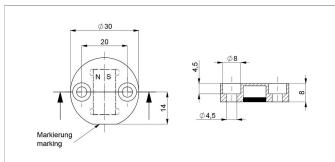
Position marker for frontal fixation with 2 cylinder head screws M4x20 (with microencapsulation, included in delivery).
