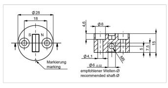
Position marker for frontal fixation with 2 cylinder head screws M4x20 (with microencapsulation) or with threaded pin M5 (both included in delivery). PF
